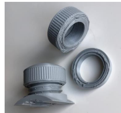
Fig 7 – Successful and unsuccessful test prints of extra fill caps and thread bosses. Own work.
