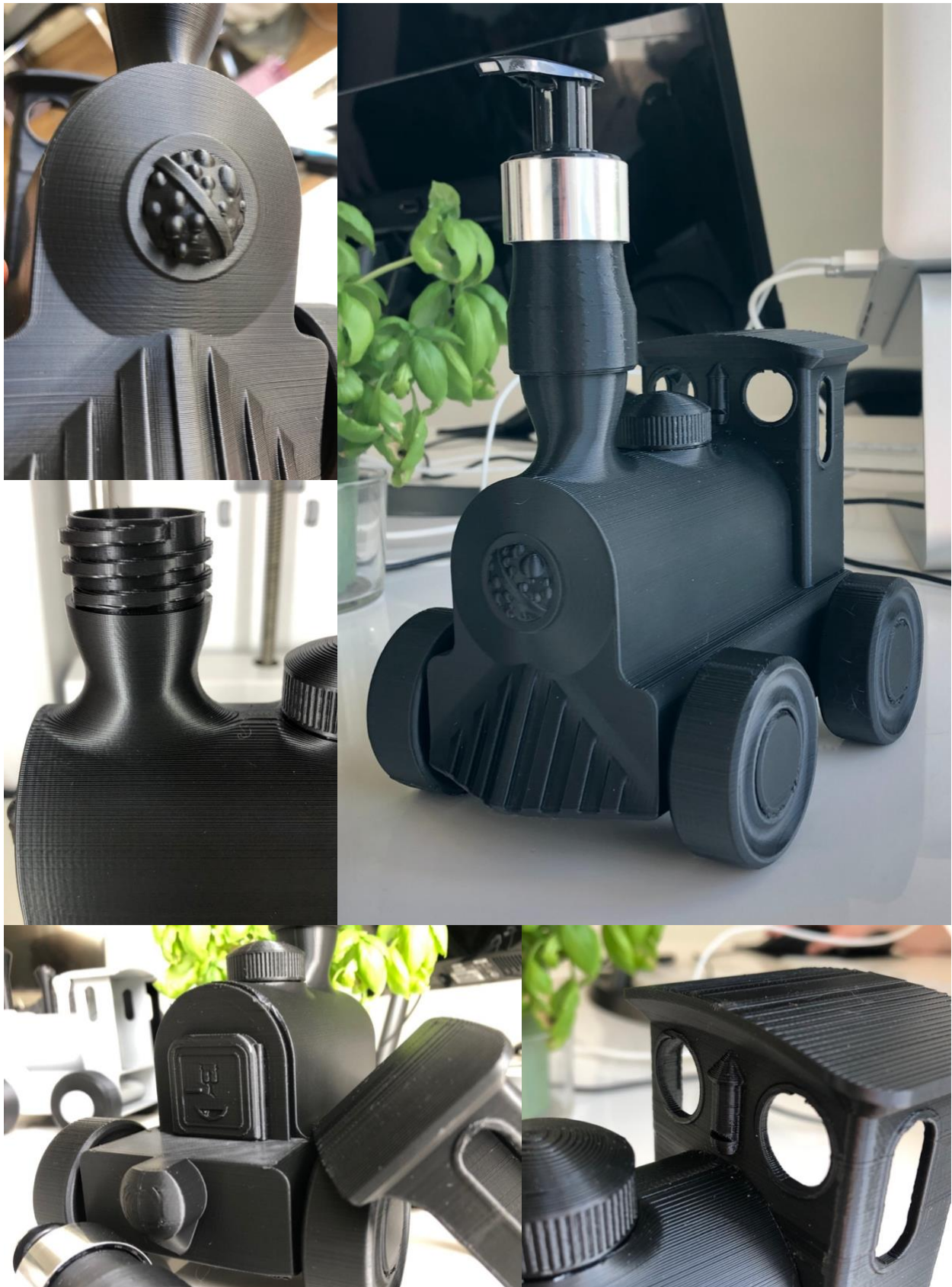
Fig 2 - Printed Lok filling all assignment requirements. Note pump not printed but salvaged from a PET bottle. Own work.
