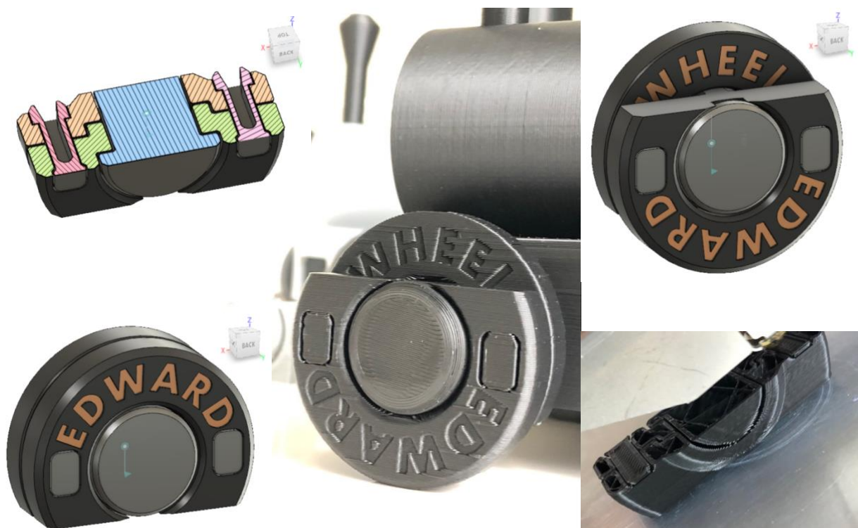
Fig 18 - Edward wheel CAD views closed, open and analysis, test and final prints. Own work. Photos and screen capture from Fusion 360 workspace.
