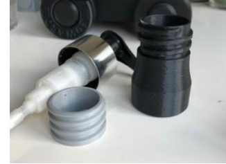
Fig 12 - Thread test, pump and stack extension.
