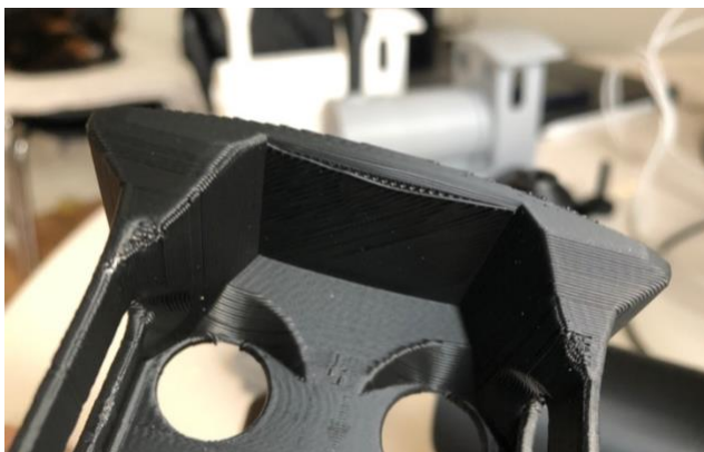
Fig 11 - Overhangs to make cabin roof printable. Note bridging and curling artifacts.
