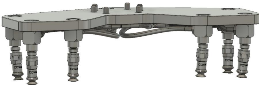
Fig 3 - Supplied end effector model for analysis. Counting all the parts involved with this assembly sums to approximately eighty and approximately eighteen of those parts are unique. Screen capture in Fusion 360 design workspace. Own work.
