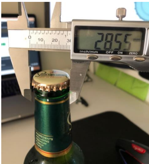
Fig 5 - Cap max width for comparison against the CAD model. Caliper raised for the photo.
