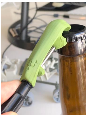
Fig 13 - First print test reveals a flaw on some harder-to-open caps. Own work. Photo of first version of opener in use.
