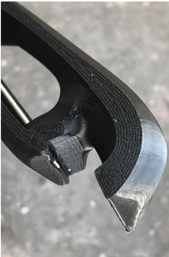
Fig 17 - Close up views of final design. Left, note screwdriver tip protruding slightly to reduce wear from the bottle cap on the opener. Right, the end of the opener deforms slightly as the screwdriver handle snaps into place. Own work.
