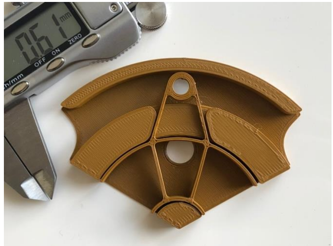
Fig 3 - Test print of 0.6 mm clearance on all vertical faces of the fixture. Spindle printed without modification from previous lesson. Own work.
